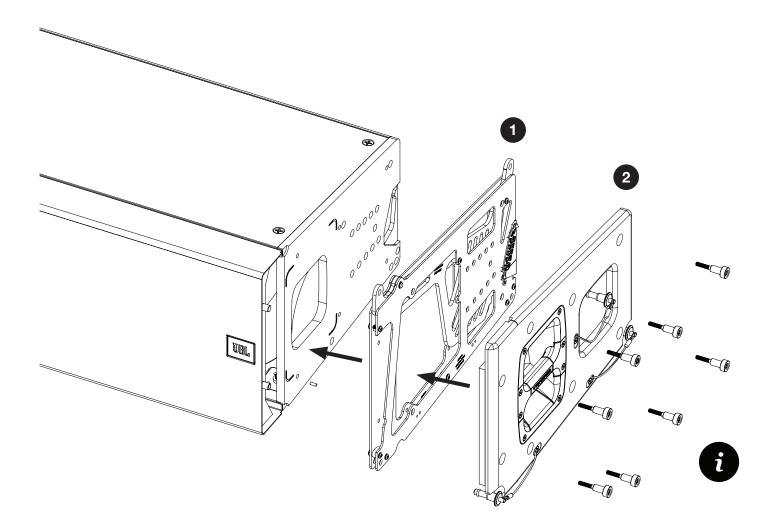
TIP: When installing the screws, take care not to damage the threads, especially when reusing the original screws, which are already coated with threadlocker. Avoid using power tools for this step.
