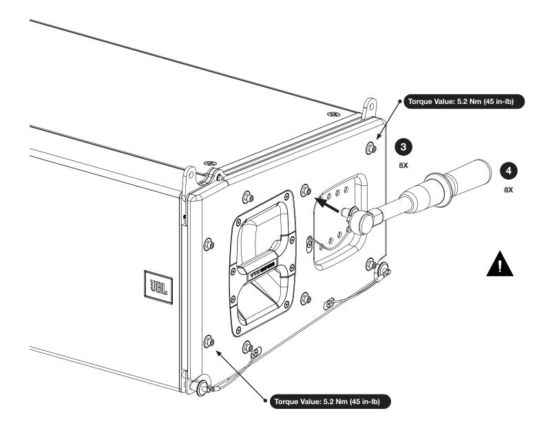
CAUTION: Apply non-permanent, medium strength threadlocker to all screws before installation. Any damaged screws should be replaced and not reused. Apply specified torque value.
